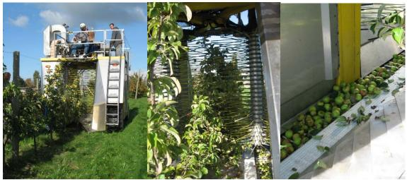
**Figure 1.** Harvesting 'Brown Snout' cider apples with an over-the-row shake-and-catch mechanical harvester at WSU Mount Vernon NWREC (left); rotating drums knock fruit off trees (center); fruit fall onto a catch plate within the harvester (right).
